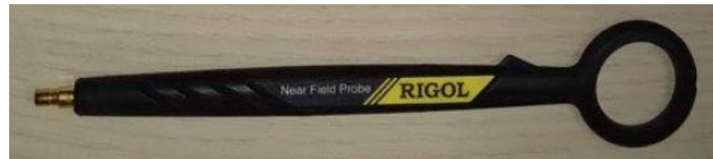
Fig: Electromagnetic Fault Injection (EMFI) Probe
